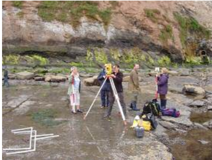
Fig.4 Setting-up the TST on one of the new 2006 datum points
