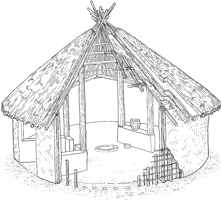
Internal cut-away of an Iron Age round house
